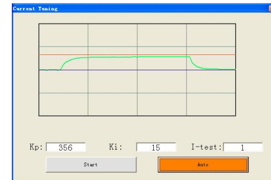
Figure 24: Kp=356, Ki=15 (poor performances)
