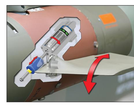
In addition to directing the missile, lead screws are used to raise missile-launching systems and deploy sighting, range-finding, and antenna equipment.
